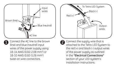
**NOTE:** For CSA approval, a disconnect/toggle switch of appropriate rating needs to be placed within 29.5 ft. (9 m) of primary side of the power supply. The minimum rating of the switch must be either 120 or 220 Volts AC. The switch must also support twice the amount of input current.
