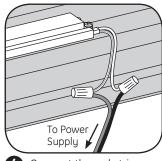
Connect the red stripe wire (+) of the LED system to the red wire (+) of the power supply. Connect the white wire (-) of the LED system to the black or blue wire (-) of the power supply.
