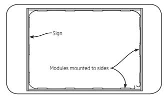
Determine location of where LED modules will be mounted based on sign dimensions (see chart). If mounting on bottom of sign, the use of a riser will be needed (minimum 1/8 in. distance between bottom surface and module).
