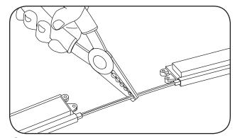
Determine how many modules are required for your application and cut where necessary.
