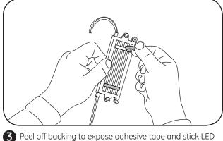
Peel off backing to expose adhesive tape and stick LED modules into place.
