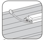
Cap all exposed wires with appropriate end caps or apply electric grade (non-conductive) silicone for additional weather protection.
