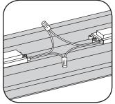
Connect modules using twist-on wire connectors or in-line (IDC) connectors. Join white wires together and red striped wires together.
