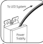
3 Run a wire from the Power Supply and connect to the first LED module on the strip.
