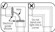
Corner: For all corners (planar, inside, outside) apply silicone on both sides to secure light guide corners. Snap on corner. Follow Steps 8-10 if wires are cut.
