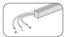
8 Separate wires and identify outer conductors as positive (+) and middle conductor as negative (-). Strip ends back 0.5 in. (13mm).
