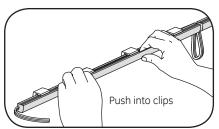
Push each 16 in. (406mm) light engine segment into the clips. Fold loose wires behind light engines. Do not stretch light engines.
