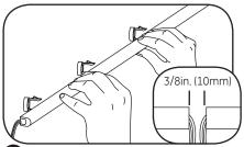
5 Attach Tetra Contour to the mounting clips, leaving a 3/8 in. (10mm) gap between sections to allow for expansion or contraction.
