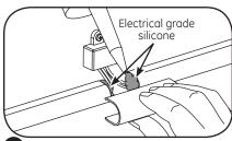
Linear: At each gap between sections, apply silicone on both sides to secure light guide connector. Snap on a light guide connector.
