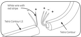
1 Tetra Contour LS can be connected to formable Tetra Contour for custom shapes. Separate wires and identify conductors as positive (+) and negative (-). Strip ends back 0.5 in. (13mm).
