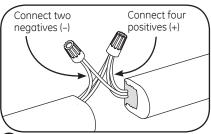
9 Use twist-on wire connectors to join wires together.
