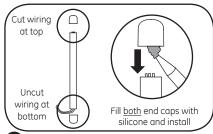
4 For vertical or near vertical installations, any cut-end termination of a Contour piece shall reside at the top of the design.
